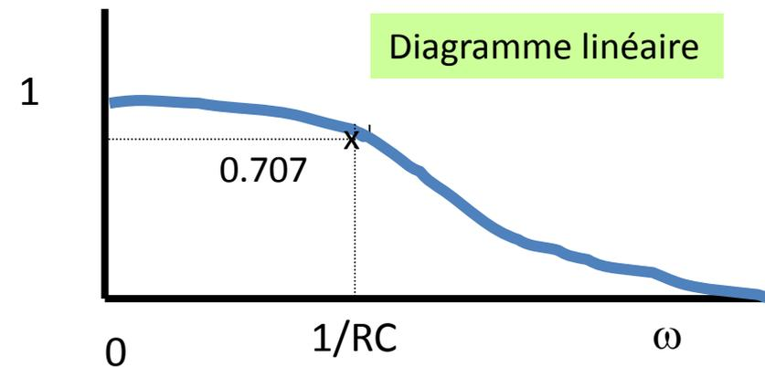
$$\frac{V_o(j\omega)}{V_i(j\omega)} = \frac{\frac{1}{j\omega C}}{R + \frac{1}{j\omega C}} = \frac{1}{1 + j\omega RC}$$
