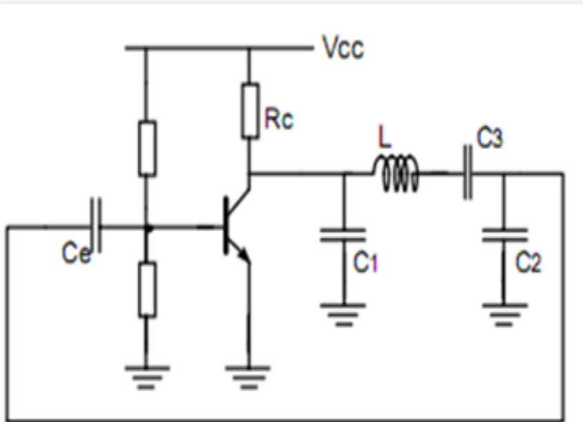
$$\omega_{osc} = \sqrt{\frac{1}{L} \left( \frac{1}{C_1} + \frac{1}{C_2} + \frac{1}{C_3} \right)}$$
