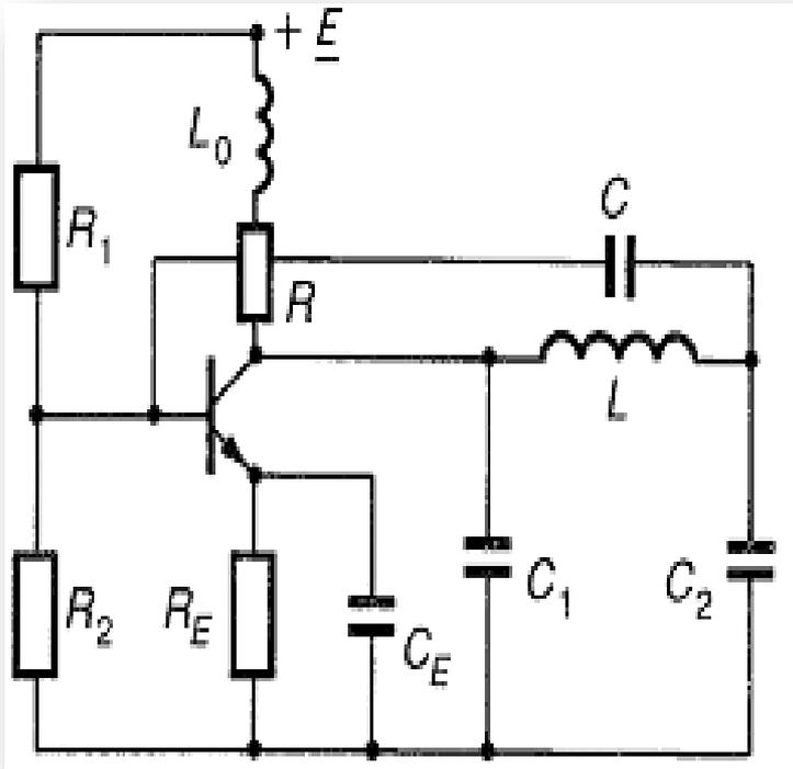
$$\omega_0 = \frac{1}{\sqrt{L \left( \frac{C_1 C_2}{C_1 + C_2} \right)}}$$
