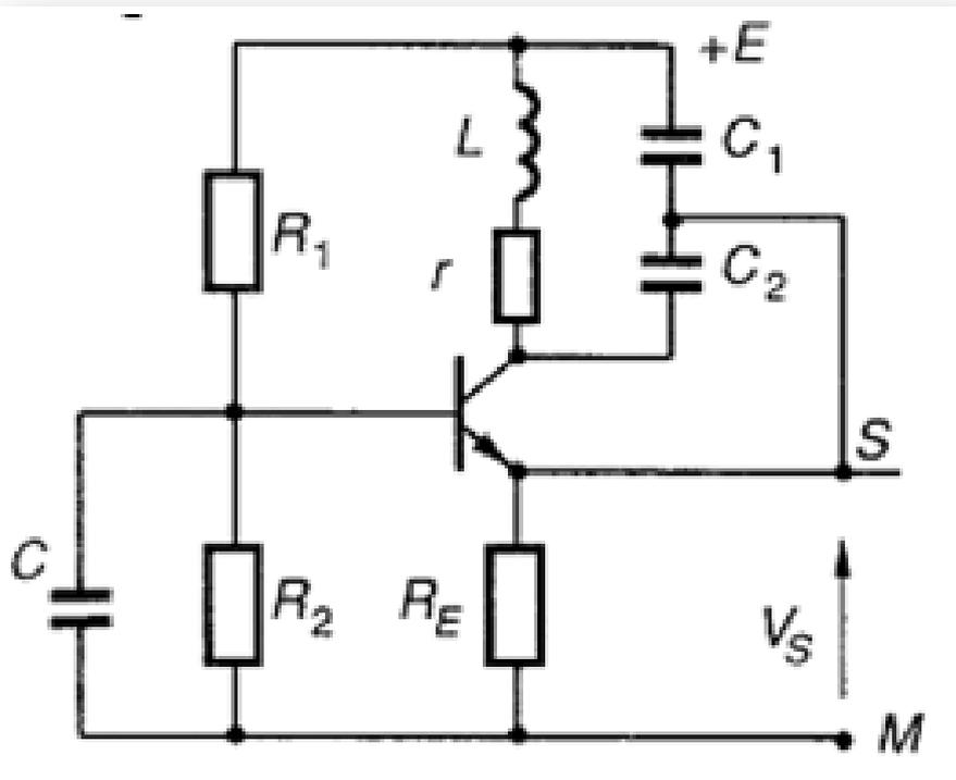
$$\omega_0 = \frac{1}{\sqrt{L \left( \frac{C_1 C_2}{C_1 + C_2} \right)}}$$
